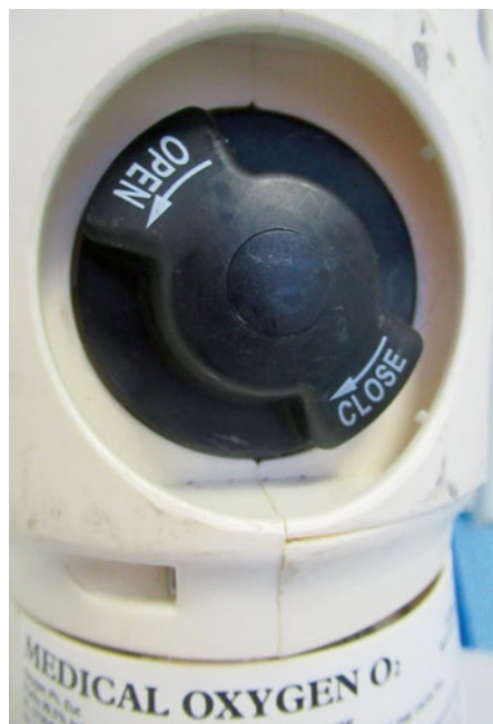
Fig. 5 An example of an integral valve on an oxygen cylinder
